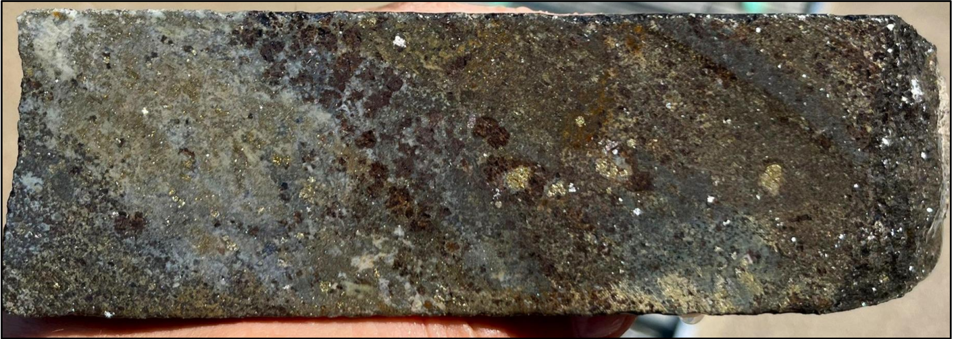
Figure 6. Skarn-hosted polymetallic mineralisation with abundant sphalerite and pyrite from 553.1m in ZRSD25189 – 0.4g/t Au, 0.3% Cu, 0.2% Pb, 6.7% Zn and 13.2g/t Ag.
