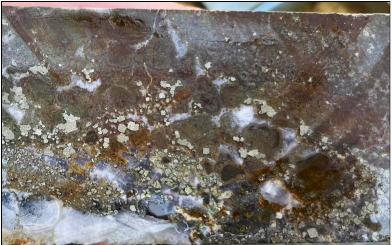
Figure 5. Skarn-hosted gold mineralisation associated with quartz-carbonate veining and disseminated pyrite from 435.3m in ZRSD25189 – 15.3g/t Au.
