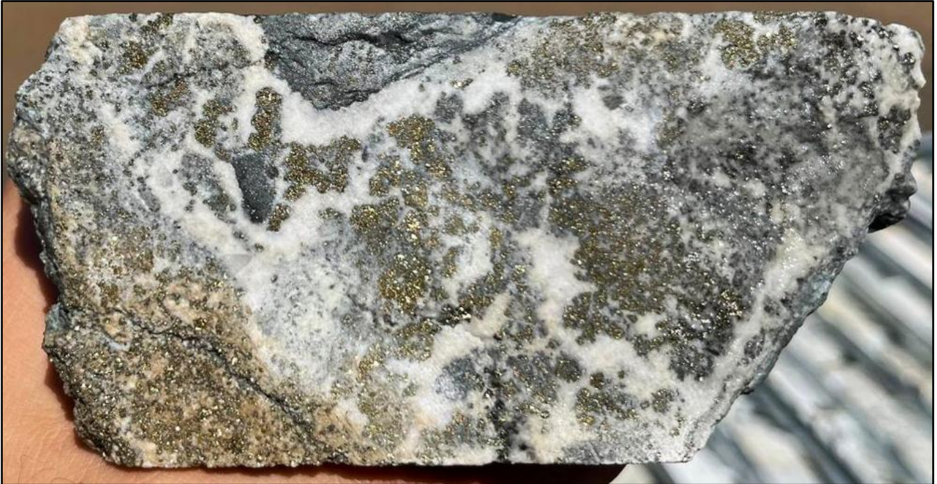
Figure 4. Skarn-hosted gold mineralisation associated with disseminated pyrite and carbonate veins from 349.4m downhole depth in ZRSD25189 – 4.4g/t Au.
