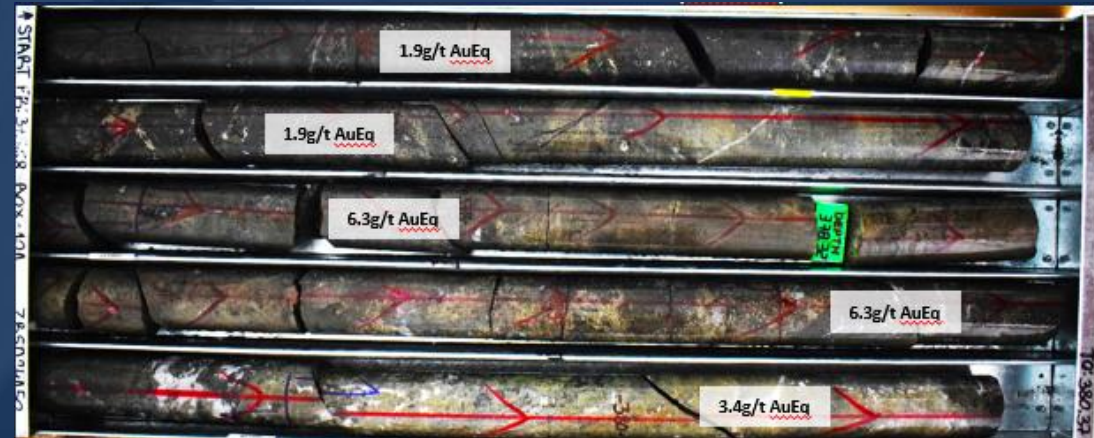
Drill core from ZRSD24150 (Shanac) 2
