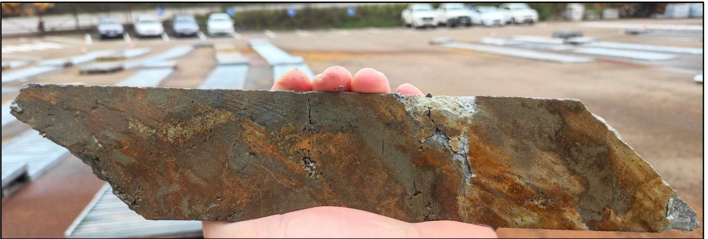
Figure 6. Photo of gold-copper-zinc mineralisation from 300.6m down-hole depth – 1.4g/t Au, 0.4% Cu, 6.6% Zn and 8.0g/t Ag.
