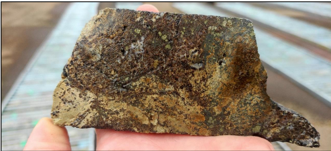
Figure 1. Photo of high-grade gold-copper-zinc skarn from 279m in ZRSD24157 – 5.4g/t Au, 1.9% Cu, 16.6% Zn and 48.9g/t Ag
