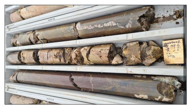
Figure 5: MWDD002 drill core (103.5 to 106.3m) showing a zone of dense (estimated 20%) boudinaged, vuggy, quartz carbonate veining with 5% ex sulphide content within the BIF saprock. This intersection is a 40m projection south from discovery hole HWAC1472.
