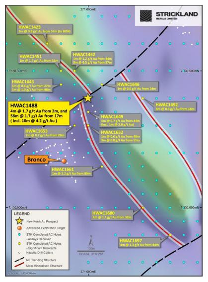
Figure 7: Topographic image showing Konik aircore anomalism
