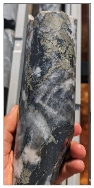
Figure 4: MRDD004 drill core (260.45 to 260.7m), showing intense quartz carbonate veining (50% quartz carbonate veining) with approximately 20% pyrite content.
