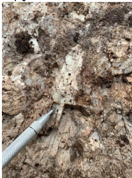
Photos 12a & 12b: Dyke #02, outcrops TR23PS-029 (left) and TR23PS-028 (right) with spodumene crystals.
