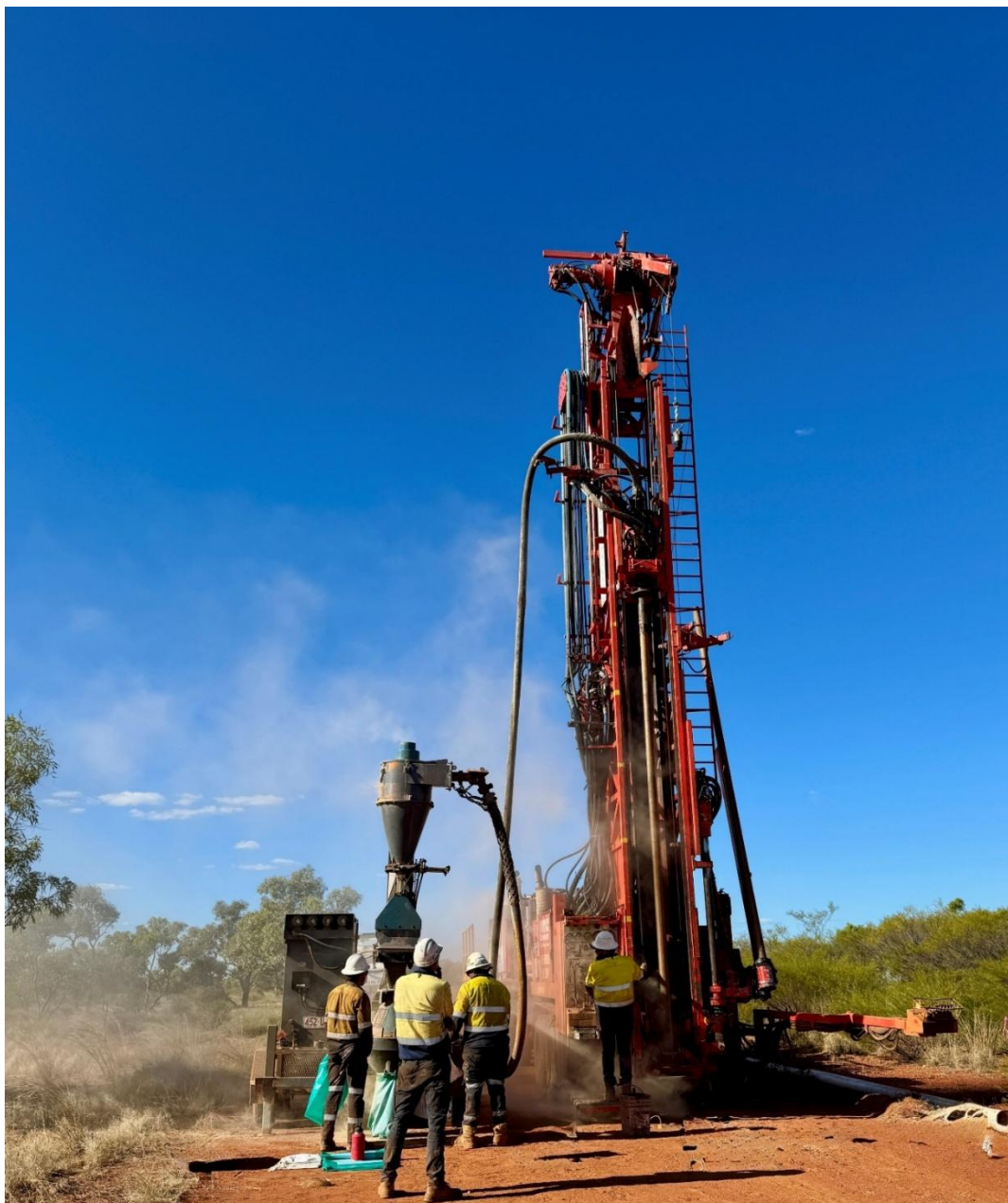
Figure 1 – RC drilling underway at the Newmans rare earth discovery, Sybella-Barkly Project, northwest Queensland.
