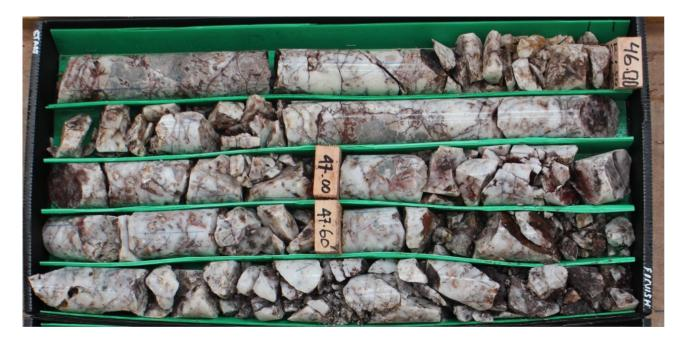
**Figure 10:** Photograph of drill core from hole APD002 showing a 3.5m intersection of near massive quartz vein and breccia. The quartz is locally chalcedonic and contains 1-3% of fine-grained disseminated pyrite.
