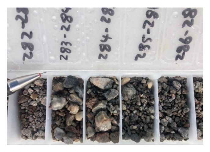
**Figure 16:** RC chips from H2RC09 which intersected a 53m stringer vein zone (241-294m), including a 3m wide quartz vein (283-286m) with crustiform textures and pyrite.
