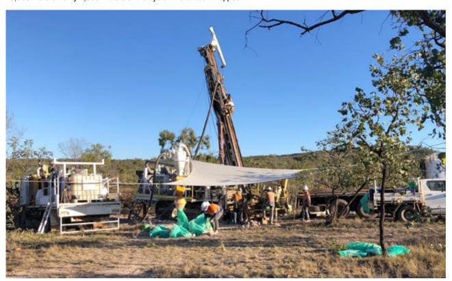
Figure 15: Photo of RC drill rig and support equipment drilling near main vein zone at Hill 212.
