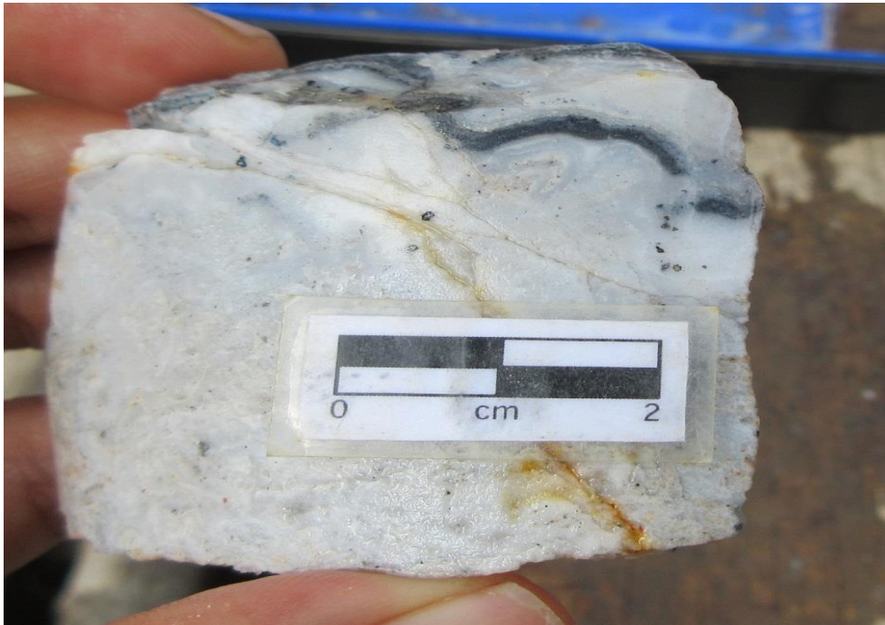
Figure 9: Image showing example of drill core sample from APD001 cut in half.
