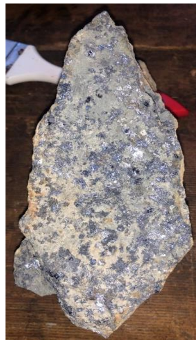
Figure 5 - Webbs Consol Main Shaft specimen showing coarse galena mineralisation
