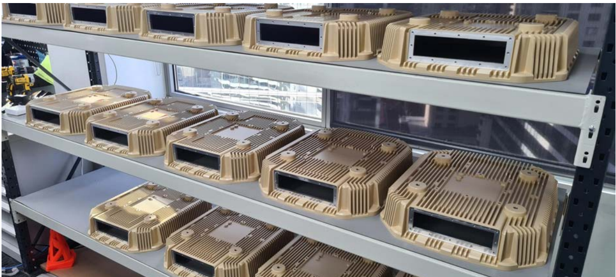
Image: DroneSentry-X™ heatsinks during the manufacturing process
