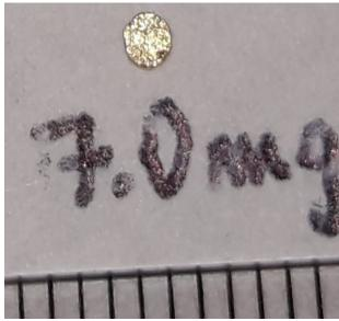
Fig. 3. Gold precipitated on copper wire from MIBK solution
