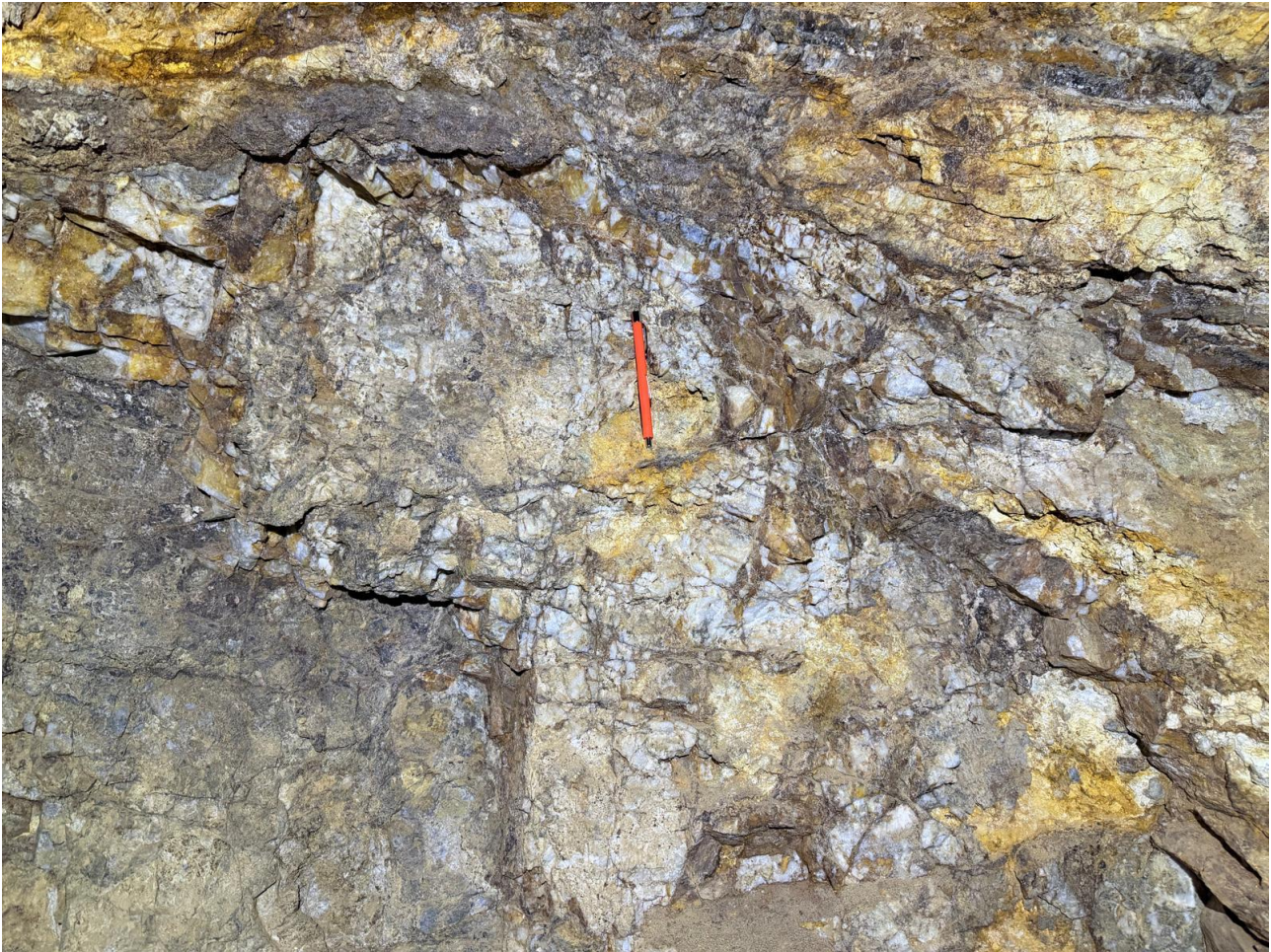
Figure 1: Shallowly dipping lode vein system from underground workings northwest of main Keystone Mine, showing oxidised, brecciated quartz veining hosting remnant sulphides and boxwork evidence of iron oxides-after sulphide.
