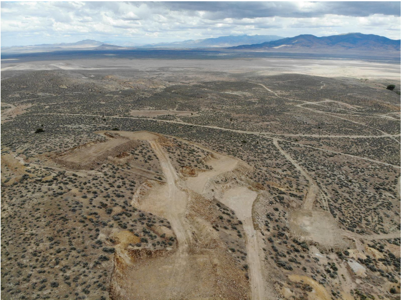
Figure 1: Aerial view of the Keystone Mine, with pads prepared for upcoming drilling campaign. Historic Keystone Mine workings can be seen in the lower left, along the north striking main Keystone Vein.
